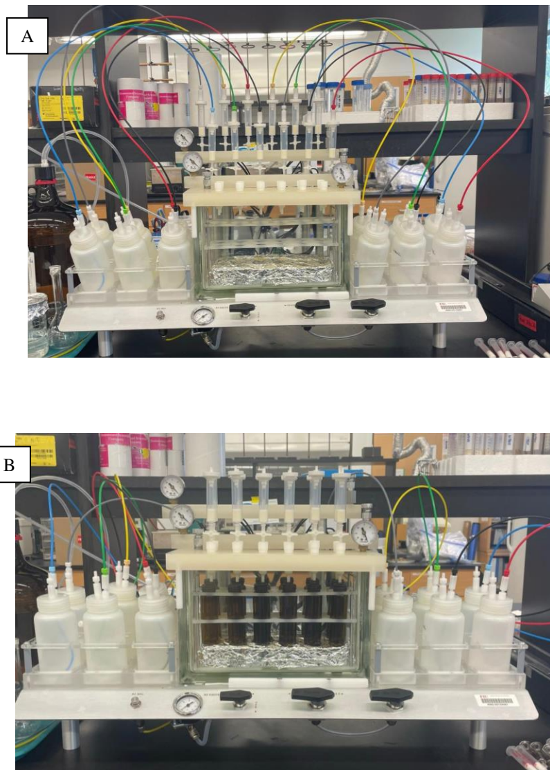
Figure 2: Semi-automated SPE equipment showing (A) stage 1- leachate samples being loaded in the cartridges and (B) stage 2- samples being eluted into 60 mL glass amber vials.
